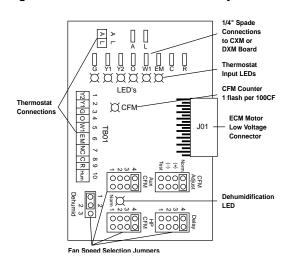
Figure 26c: ECM Version III Interface Layout
